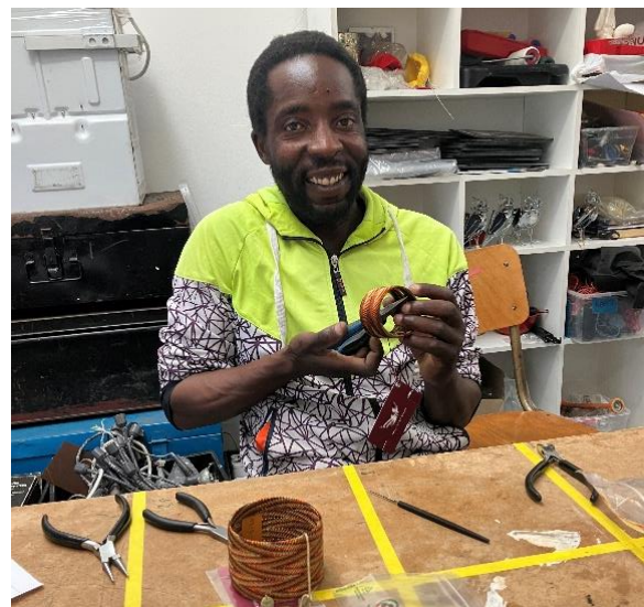
Felix Mukuze of African Robots, in Cape Town, at work hallmarking all the Threads bowls and bangles, using little discs that have the logo, weaver’s name and year, metal content and unique number.
