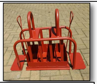
If this maker is not available these blocks can be pressed by hand into plastic containers of appropriate size.
